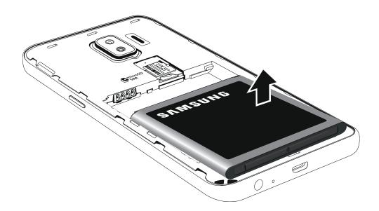
Remove the battery from the device.
