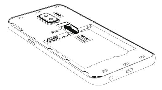
2. Slide the memory card into the slot with the gold contacts facing down.
